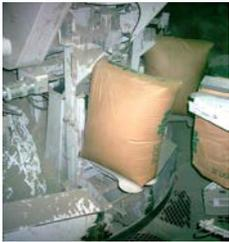
Controlling the flow of cement to the bagging area allows for better productivity and downtime. Kinetrol positioner assemblies allow for cement flow to be accurately regulated. Kinetrol units are also installed on automated cement sampling units ensuring consistent quality.
